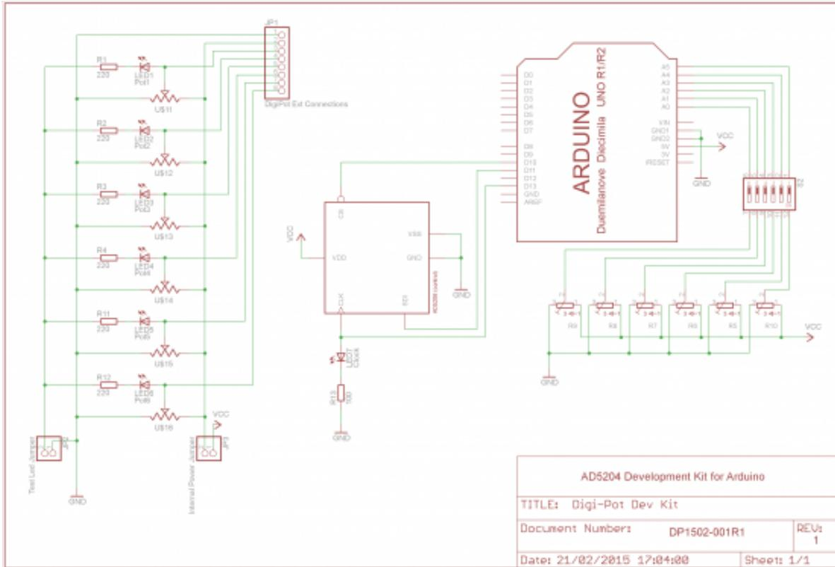
There are 6 trimmers connected to the 6 analog PINs on the Arduino board to be used for testing purposes or to generate an analog predefined value (e.g. as a preset level for the microcontroller Sketch). The triggers can be excluded one by one through the dip switch freeing the corresponding Analog PIN for other usages.
